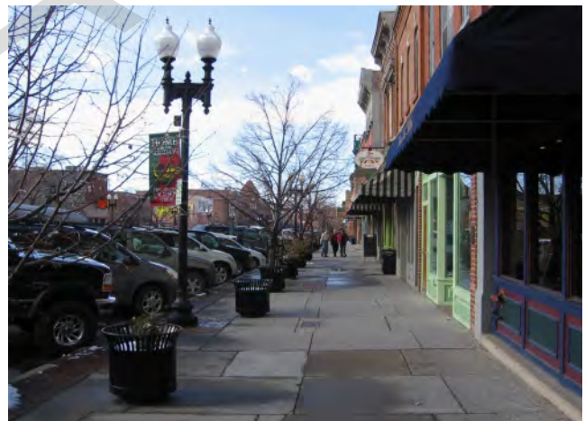
Sidewalk on 25th St in Ogden separated from traffic by trees, planters, and parking
