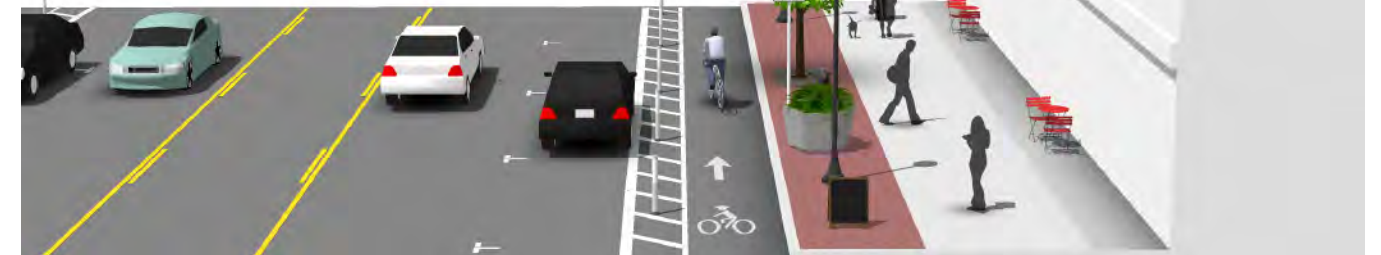
Paint and bollard street-level protected bike lane retrofit:
