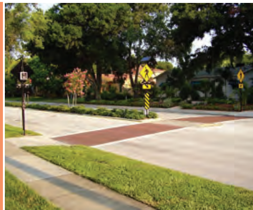
Brick RRFB-controlled crossing in a school zone (Photo: Safe Routes to School Coalition)
